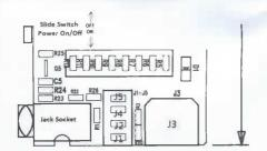
NB Additional Doors/Windows can be monitored using extra sensor sets with a single transmitter. If more than one pair of magnetic sensors are used, wiring of the sensors to the internal terminal block must be in series
